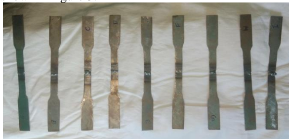
Fig.3-welded specimens for tensile test.
